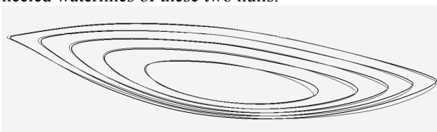
Figure 7: Heeled waterlines of hulls 0 (black) and 4 (grey).
