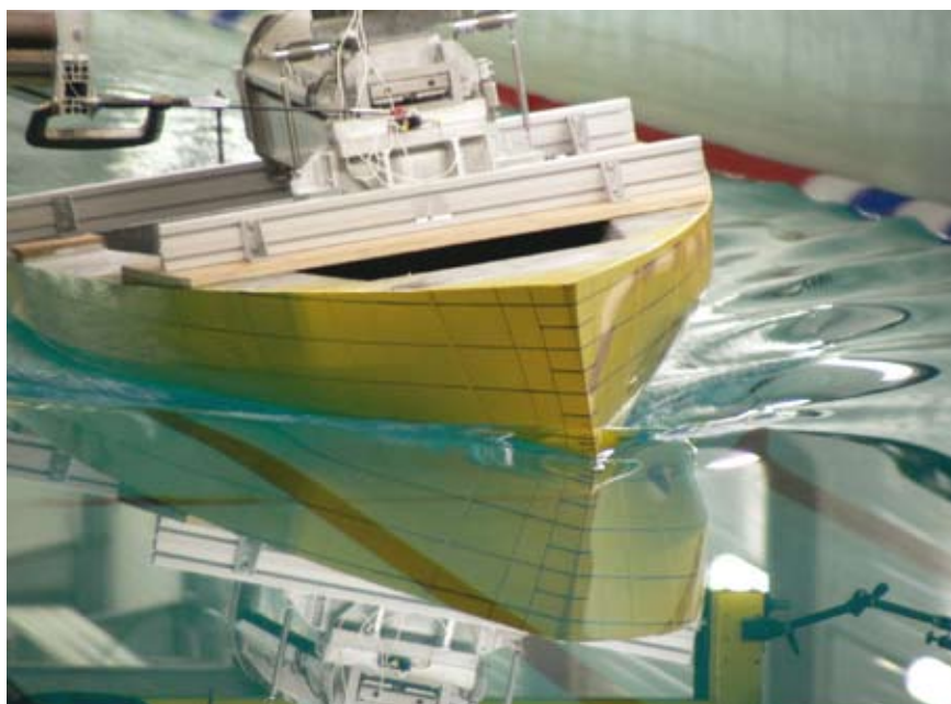
Tank testing the Groupe Finot Open 60 (as used on Generali ) the parent hull for Raymond's systematic series (Credit: Jérémie Raymond).
